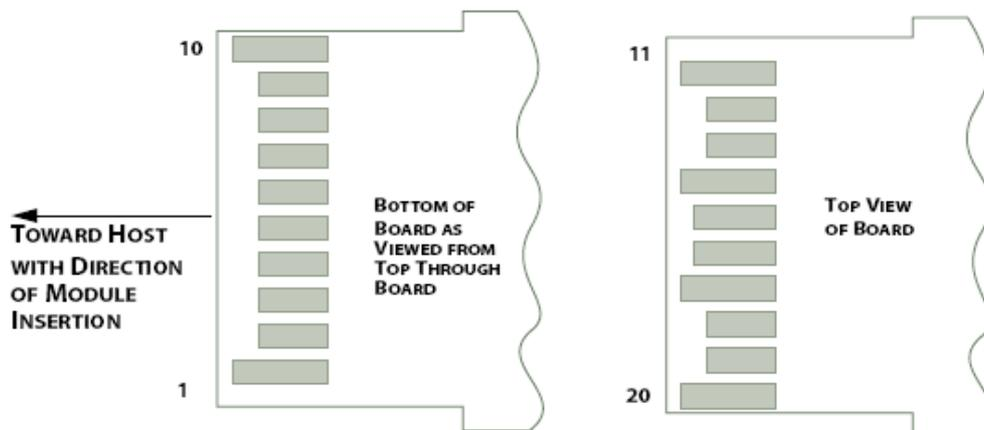
◆ Figure 3: Module Contact Assignment
